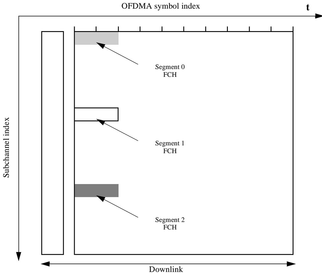
**Figure 220—FCH subchannel allocation for all 3 segments**
