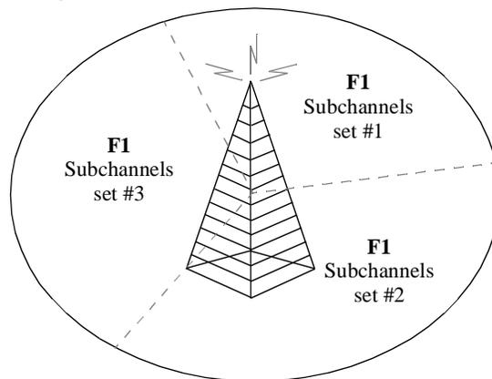
**Figure B.6—Reuse of 1 configuration, 3 sectors per cell**
