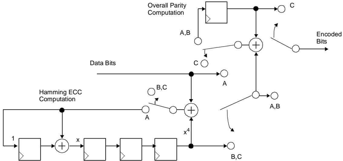
**Figure 149—Example encoder for a (16,11) extended Hamming Code**
