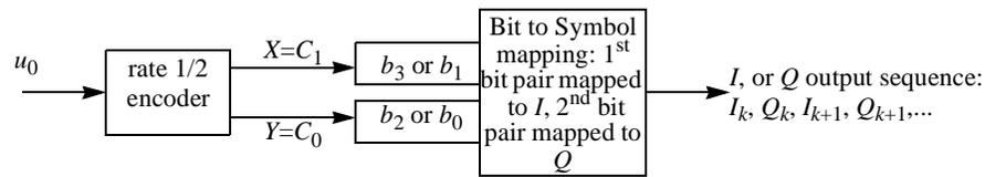
Figure 162—Pragmatic TCM encoder for rate 1/2 16-QAM
