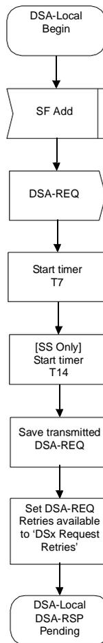
Figure 106—DSA—Locally Initiated Transaction Begin state flow diagram
