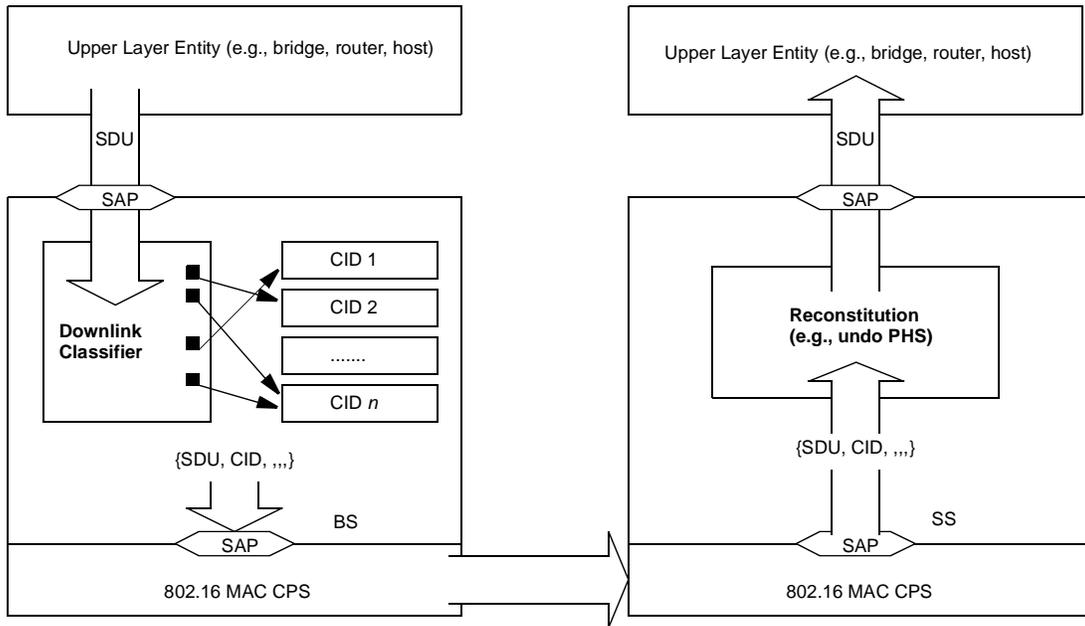
**Figure 7—Classification and CID mapping (BS to SS)**
