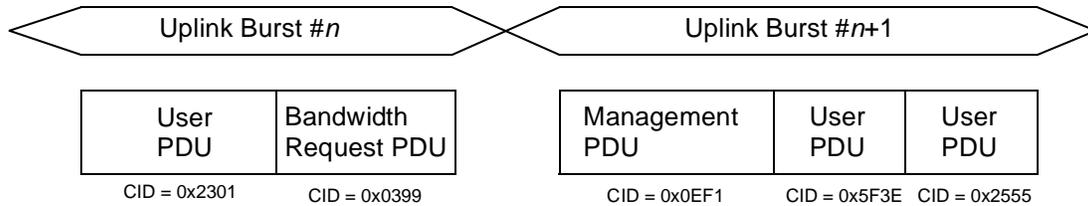
**Figure 25—MAC PDU concatenation showing example CIDs**
