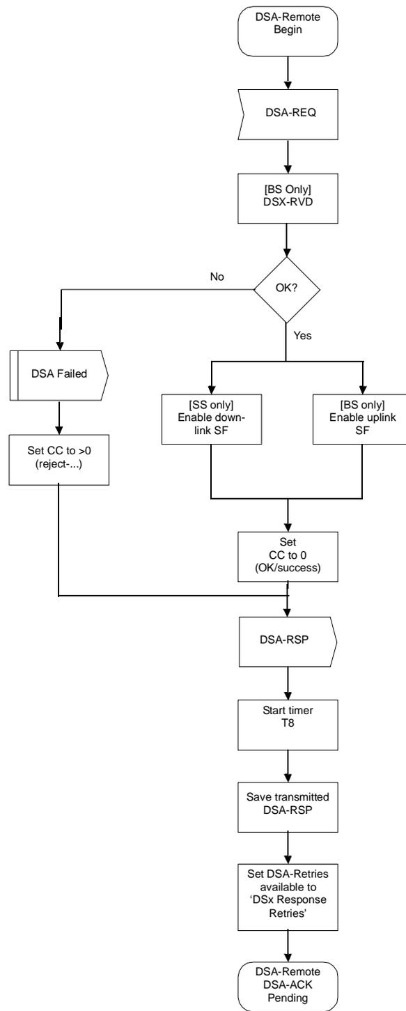
Figure 111—DSA—Remotely Initiated Transaction Begin state flow diagram
