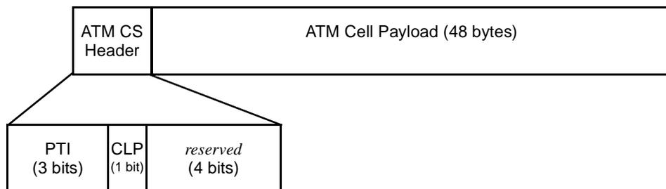
Figure 5—CS PDU format for VC-switched ATM connections
