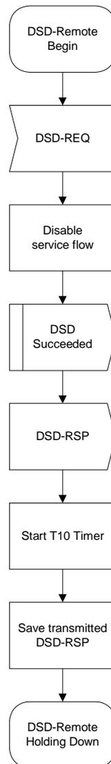
Figure 127—DSD—Remotely Initiated Transaction Begin state flow diagram
