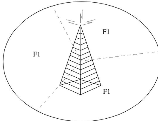
Figure B.5—Reuse of 1 configuration, 3 sectors per cell
