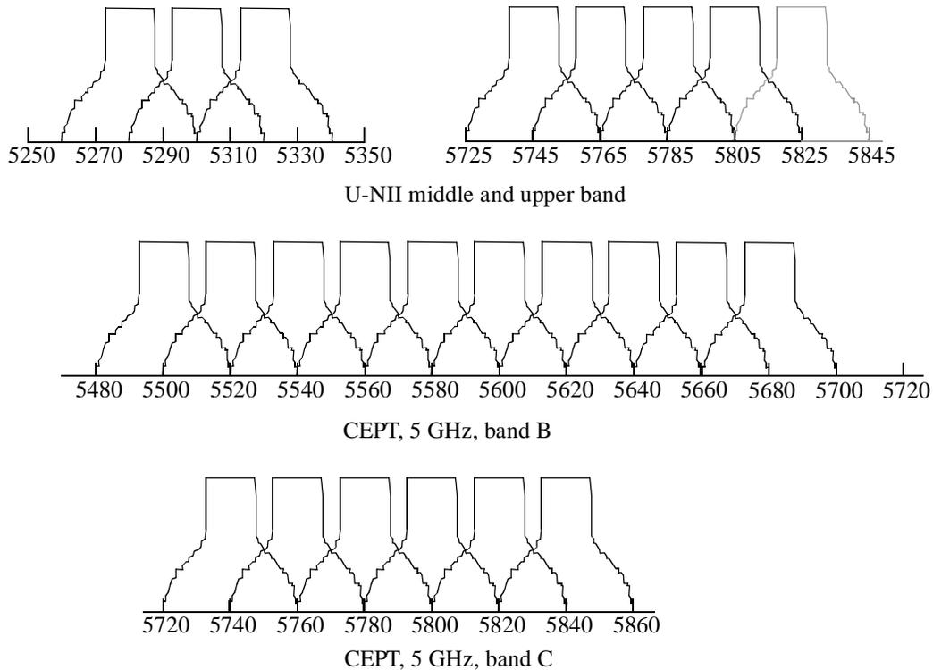
**Figure 264—Channelization, 20 MHz**
