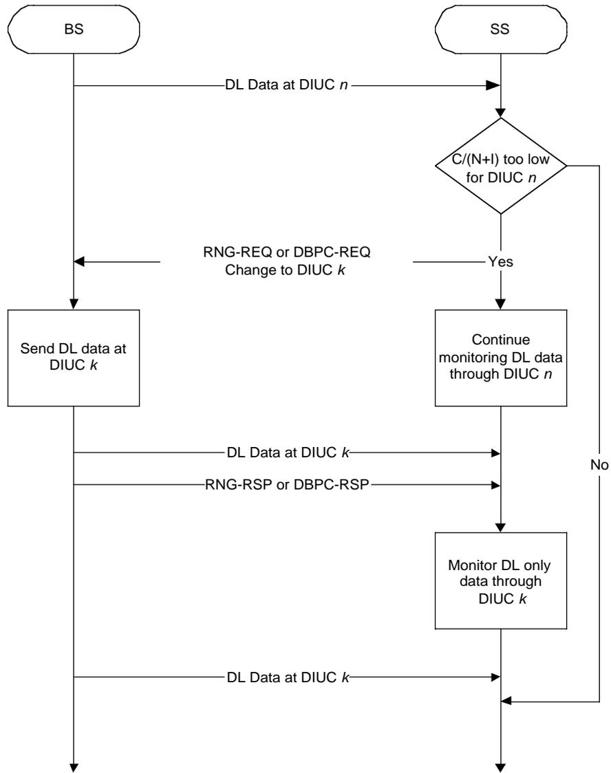
**Figure 79—Transition to a more robust burst profile**
