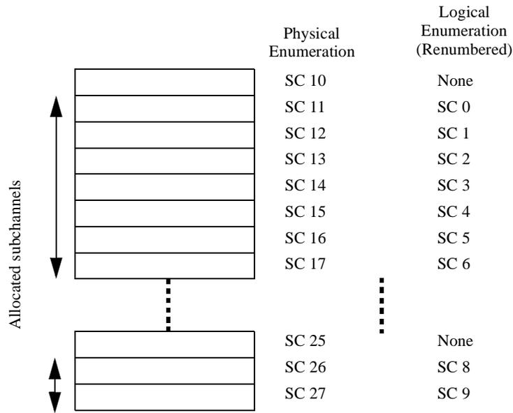
**Figure 222—Example of UL renumbering the allocated subchannels for segment 1 in PUSC**
