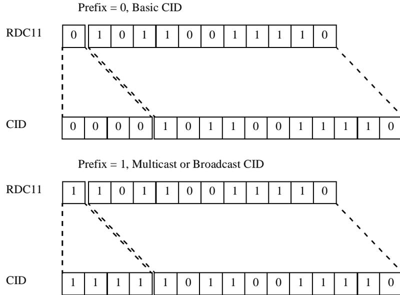
Figure 22—Reduced CID Decoding
