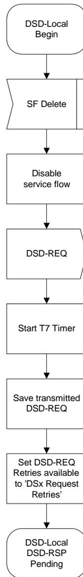
Figure 124—DSD—Locally Initiated Transaction Begin state flow diagram
