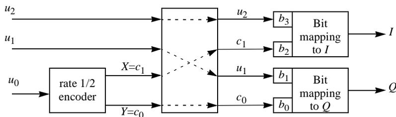
Figure 163—Pragmatic TCM encoder for rate 3/4 16-QAM
