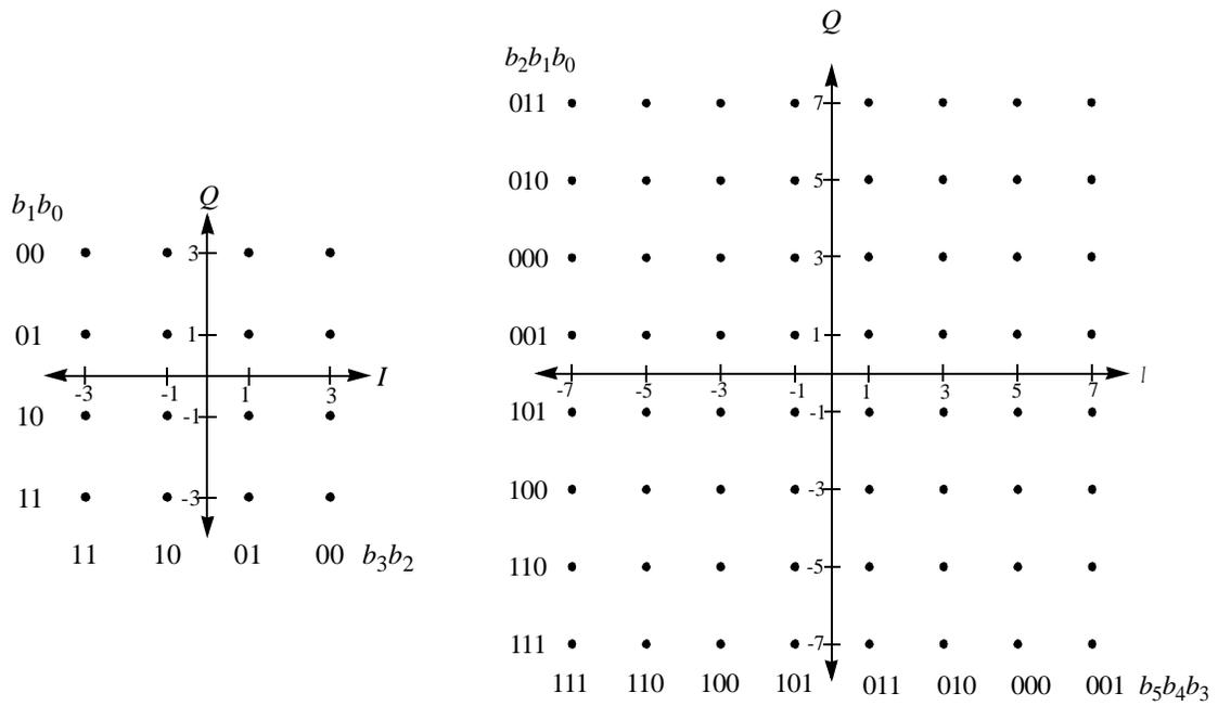
Figure 174—Pragmatic maps for 16-QAM and 64-QAM constellations
