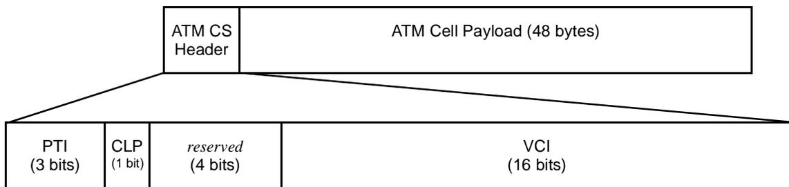
Figure 4—CS PDU format for VP-switched ATM connections
