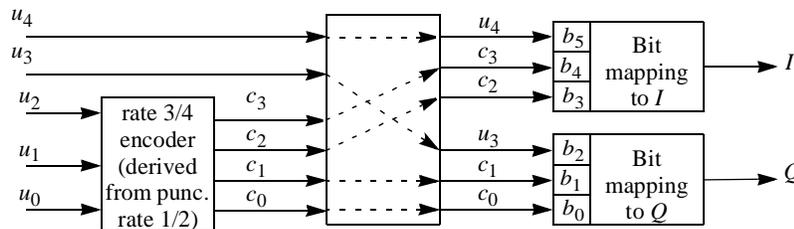
Figure 165—Pragmatic TCM encoder for rate 5/6 64-QAM
