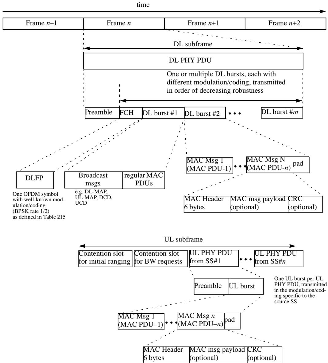
Figure 208—Example of OFDM frame structure with FDD
