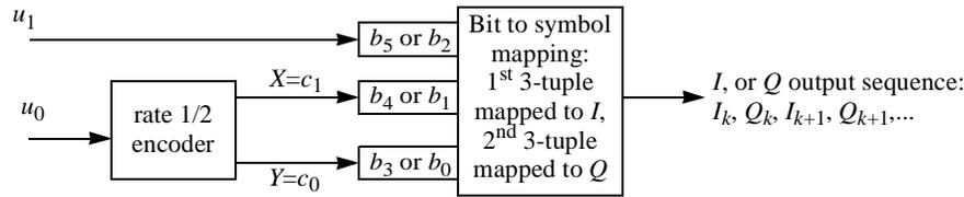
Figure 164—Pragmatic TCM encoder for rate 2/3 64-QAM
