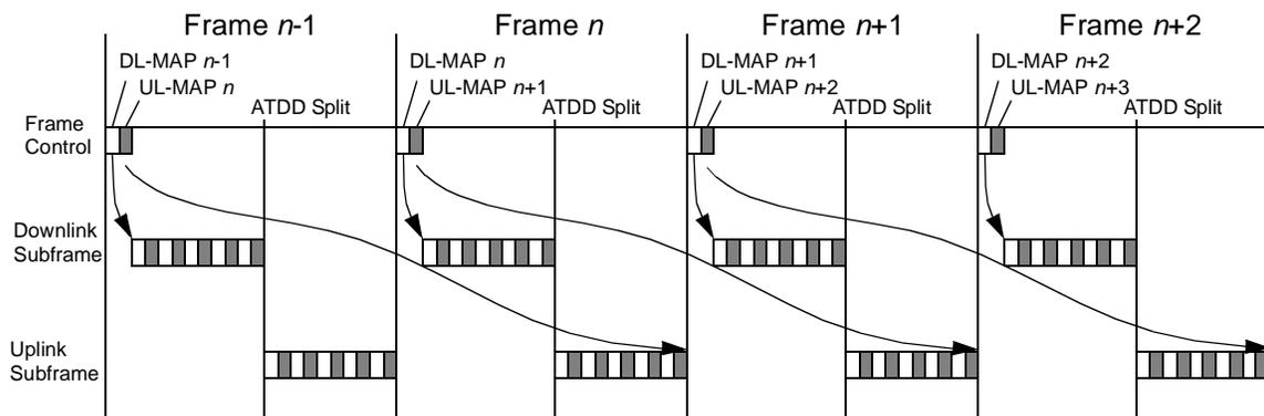
Figure 46—Maximum time relevance of DL-MAP and UL-MAP(TDD)
