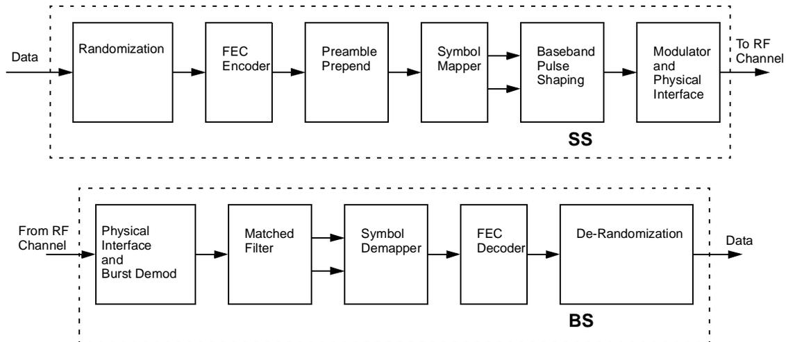
Figure 155—Conceptual block diagram of the uplink PHY
