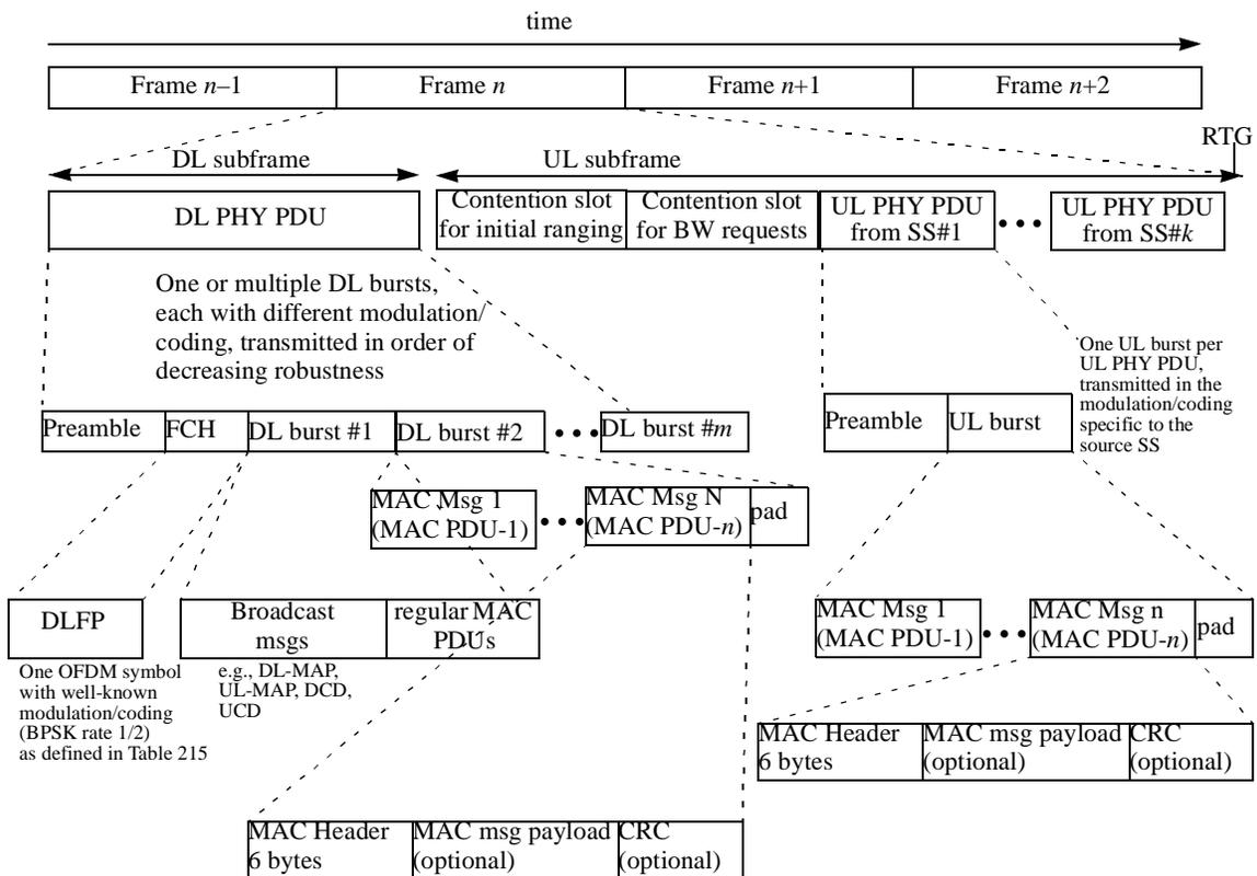
Figure 207—Example of OFDM frame structure with TDD
