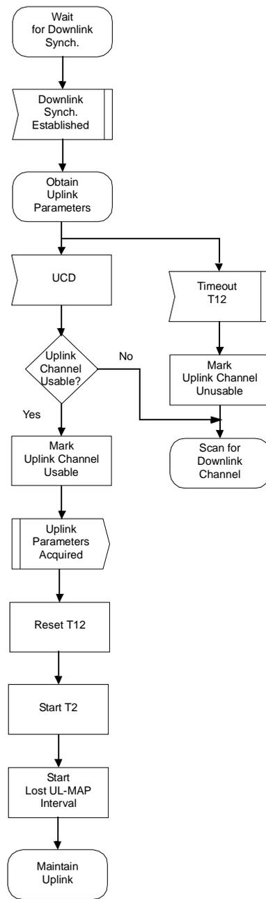
Figure 58—Obtaining uplink parameters
