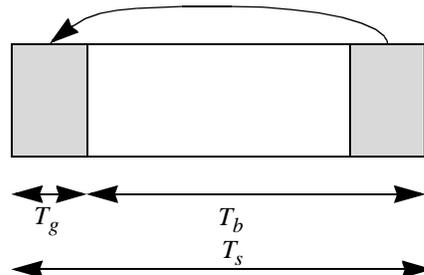
Figure 213—OFDMA symbol time structure
