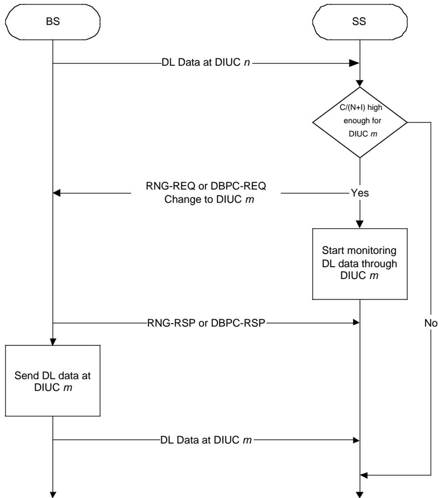
Figure 80—Transition to a less robust burst profile
