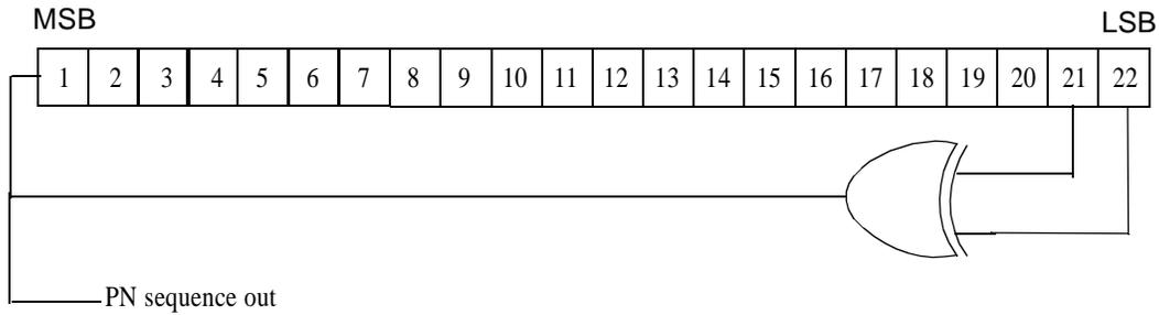
**Figure 177—Spreading PN sequence generator**
