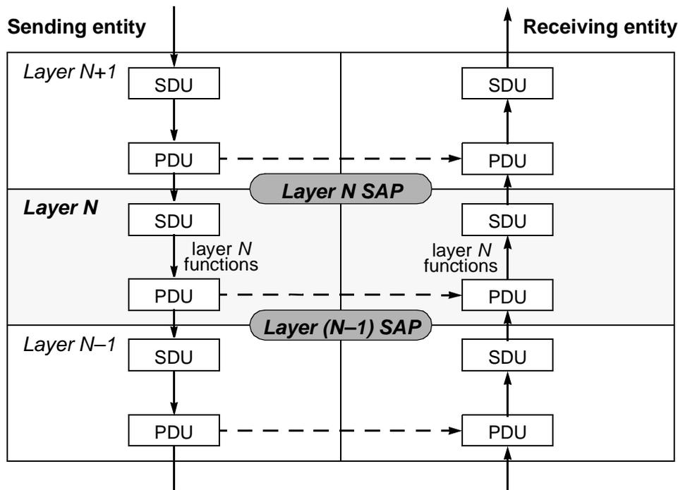
Figure 2—PDU and SDU in a protocol stack
