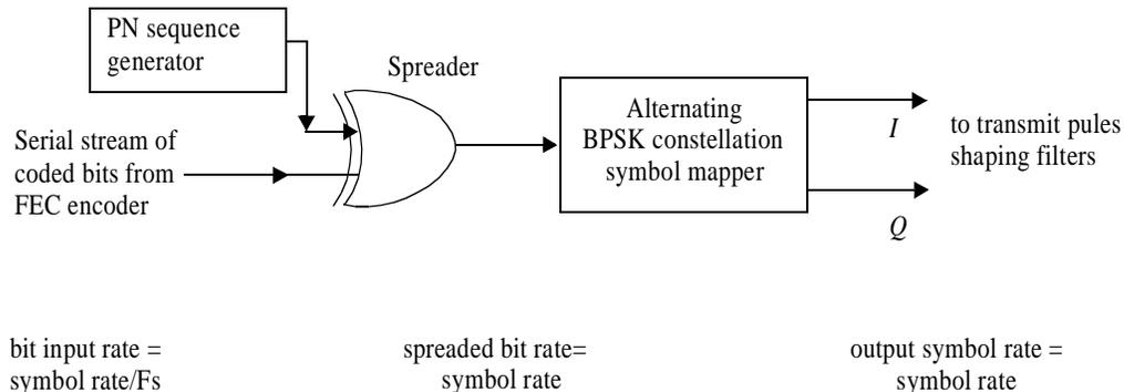
**Figure 176—Spread BPSK processing**
