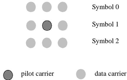
**Figure 237—Description of an uplink tile**
