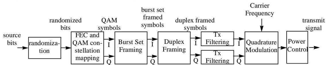
**Figure 158—Transmit processing**
