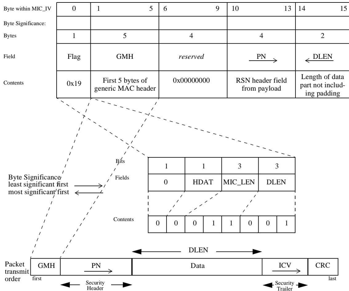
**Figure 136—Initial CCM Block B<sub>0</sub>**
