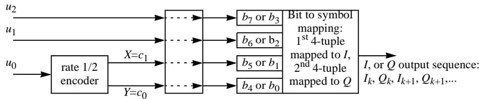
Figure 166—Optional pragmatic TCM encoder for rate 3/4 256-QAM
