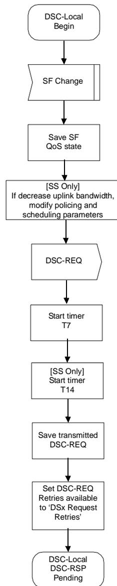
Figure 115—DSC—Locally Initiated Transaction Begin state flow diagram
