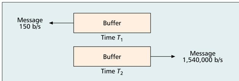
■ **Figure 3.** The time transformer concept in packet switching.
